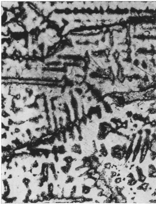
Figure 1 Nb 3 Al, containing 23 at. % Al, showing the dendritic structure, \times 80 .
